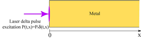
FIG. 1. (Color online) Schematic of the metal being excited by a laser delta pulse at its free top surface ( x=0 ).
